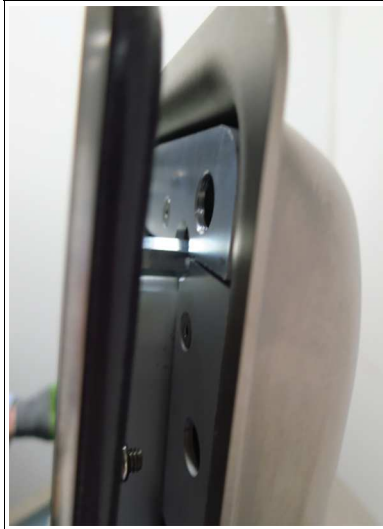
Figure 3.19 Display panel bolts lined up with the cutout holes on the inner frame
