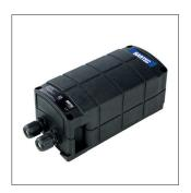
The supply module Ex i is designed for an intrinsically safe supply (barrier) of the corded hand-held scanner BCS 3608ex-IS and contains a safety barrier (evaluation barrier) for data lines in a potentially explosive atmosphere. The data cables can be connected in hazardous areas to systems – for example to HMI, PLC or micro processors, with corresponding Ex i interface- without any additional barrier/safety barrier.
