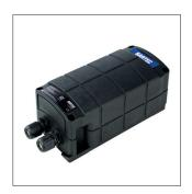
The supply module Ex i is designed for an intrinsically safe supply (barrier) of the Bluetooth hand-held scanner BCS 3678 $^{\mbox{\tiny ex}}$ -IS and contains a safety barrier (evaluation barrier) for data lines in a potentially explosive atmosphere. The data cables can be connected in hazardous areas to systems – for example to HMI, PLC or micro processors, with corresponding Ex i interface- without any additional barrier/safety barrier.
