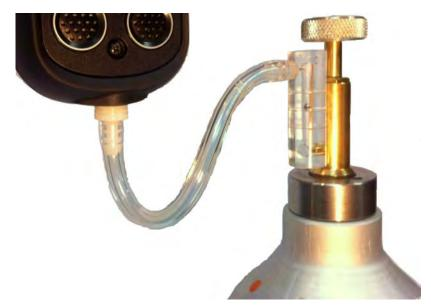
Figure 6-4: Bump Test Kit
