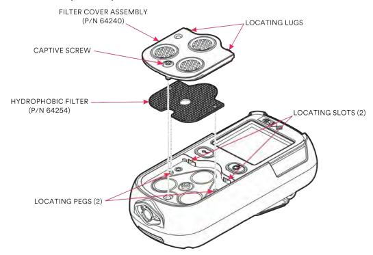
Figure 8-1: Hydrophobic Filter Replacement
