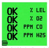
Figure 2-4: OK Display Example (4-Gas)
