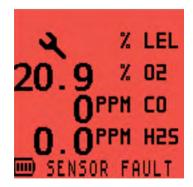
Figure 5-6: LEL SENSOR FAULT
