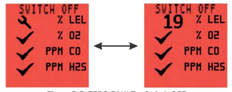
Figure 5-5: ZERO FAULT - Switch OFF
