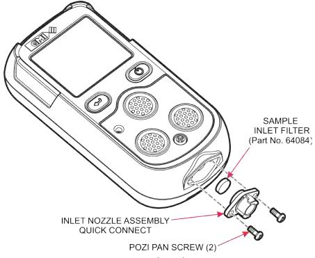
Figure 8-2: Sample Inlet (Dust) Filter Replacement
