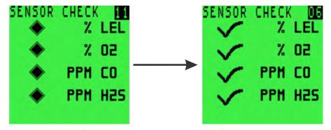
Figure 3-12: Sensor Check Displays
