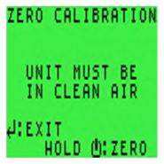
Figure 9-2: ZERO CALIBRATION Screen
