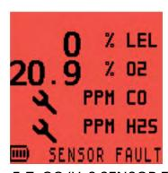
Figure 5-7: CO/H<sub>2</sub>S SENSOR FAULT
