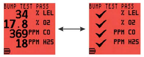
Figure 6-6: Bump Test Pass
