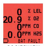
Figure 5-2: BAT FAULT Warning
