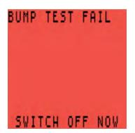
Figure 6-8: Bump Test Fail - Switch Monitor OFF
