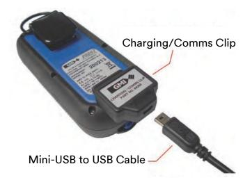
Figure 7-2: Connect Cable to Charging/Comms Clip
