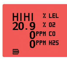
Red display in alarm conditions
