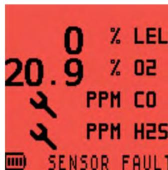
Figure 5-7: CO/H<sub>2</sub>S SENSOR FAULT
