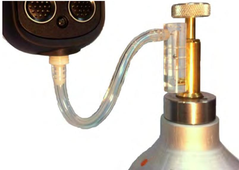
Figure 6-4: Bump Test Kit
