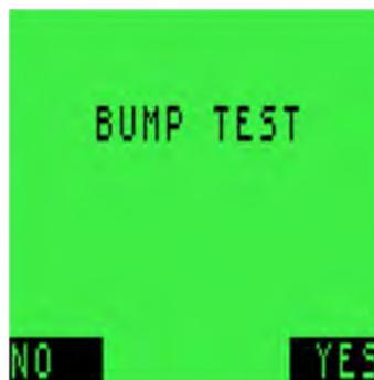
**Figure 6-1: BUMP TEST Confirmation Screen**
