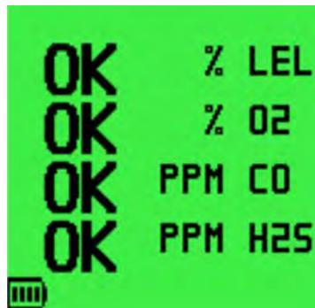
Figure 2-4: OK Display Example (4-Gas)
