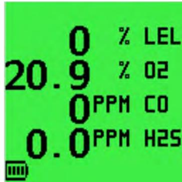
Figure 3-13: 4-Gas Normal Operating Display
