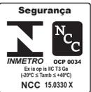
CLASS I DIV 1 GRPS A-D T3 Ex ia op is IIC T3 Ga
