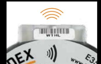
Embedded RFID chip enables open-architecture databasing with any compatible RFID enabled device. Use with CorDEX CONNECT enabled imagers for automatic transmission correct and reporting
